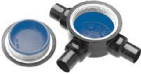
GUA series conduit bodies are installed within hazardous area locations to protect conductors in threaded rigid conduit, act as pull and splice boxes, provide access to conductors for maintenance and future system changes, act as mounting outlets for fixtures (with proper covers), or change conduit direction.
