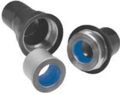
UNY and UNF unions are installed in threaded thick-wall conduit systems in hazardous areas. UNY unions are used to connect conduit to a conduit fitting, junction box, or device enclosure. UNF unions are used to connect conduit to conduit, or to provide a means for future modifications to the conduit system.
