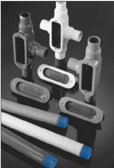
Specify OCAL-BLUE coating wherever the environment is corrosive... OCAL-BLUE is a dense polyvinyl chloride coating with a minimum thickness of 0.04" (40 mil) on the exterior and a chemically-cured blue urethane coating with a nominal thickness of .002" (2 mil) on the interior and over the hot dipped galvanized threads.
