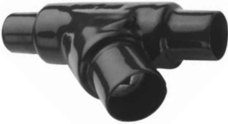
Sealing fittings restrict the passage of gases, vapors, or flames from one portion of the electrical installation to another at atmospheric pressure and normal ambient temperatures. They prevent precompression or “pressure piling” in conduit systems.
