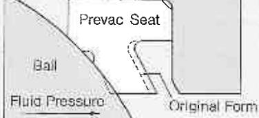
\*The downstream seal is flexibly sealing according to a fluid pressure as illustrated above.
