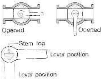
The lever mounted in two directions will cause an open and close of the valve be reversed, if wrongly installed.
