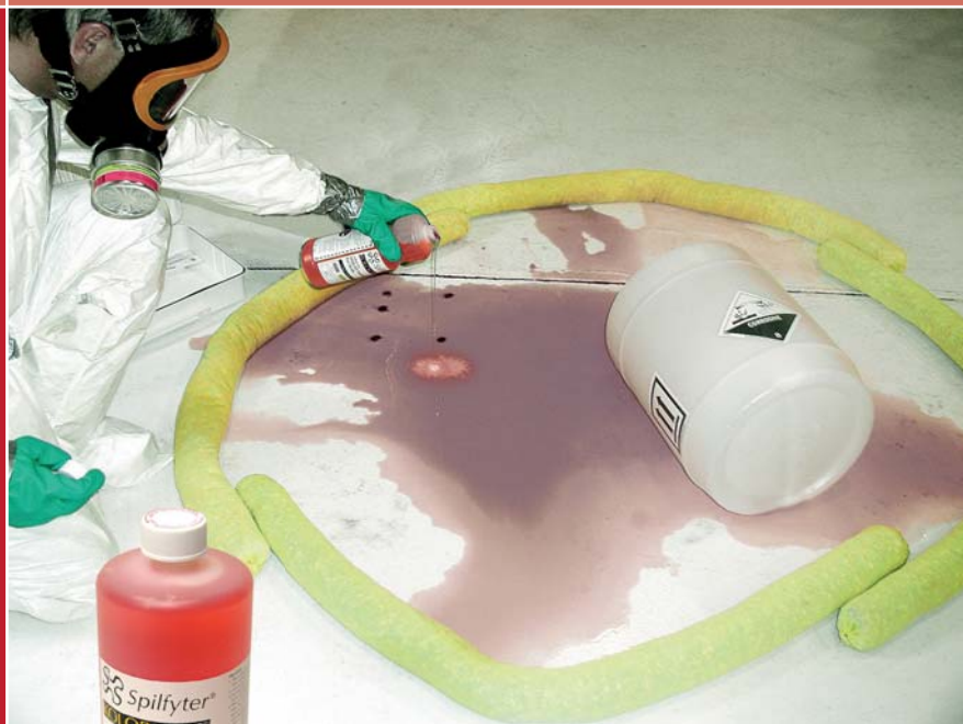
▲ Liquid Formula Generates Less Gas and Heat During Neutralization then Dry Formula
