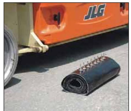
Rolled up Scissor Lift Diaper and Fastening Magnets
