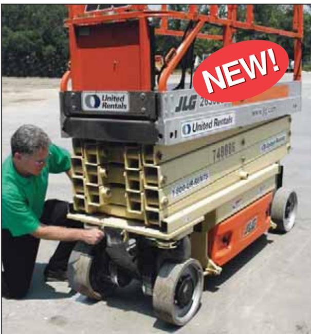
Final stages of installation — centering Scissor Lift Diaper and securing with included Fastening Magnets.
