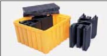
Inner polyethylene supports feature a dense pattern of vertical ribs which provide superior strength. Rated at 16,000 lbs. UDL capacity, the Ultra-IBC Spill Pallet will provide years of service under rigorous conditions.
