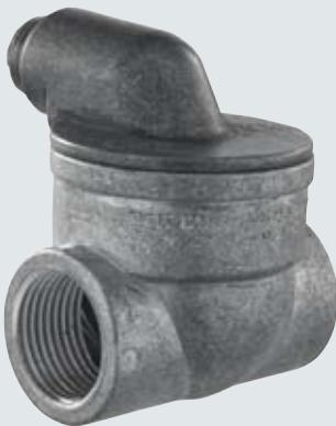
Sealing fittings prevent the passage of gas, vapors or flames through pipes system. EYS series vertical fittings are available in two different dimensions: the first up to 1"; the second up to 3" with an additional lateral opening for easy insertion of glass-fiber. EZS series are used for both vertical and horizontal mounting.
