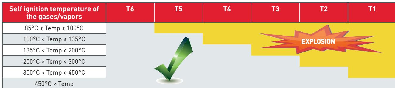
Equipment must never be used in an atmosphere capable of ignition at the temperature indicated on the marking (temperature class).
