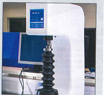
measuring hardness of the striking face
