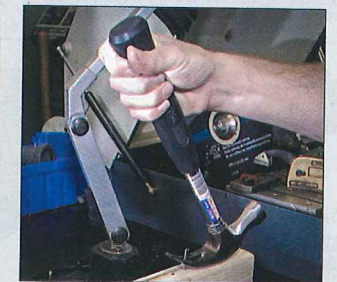
Nail extraction test for claw hammer
